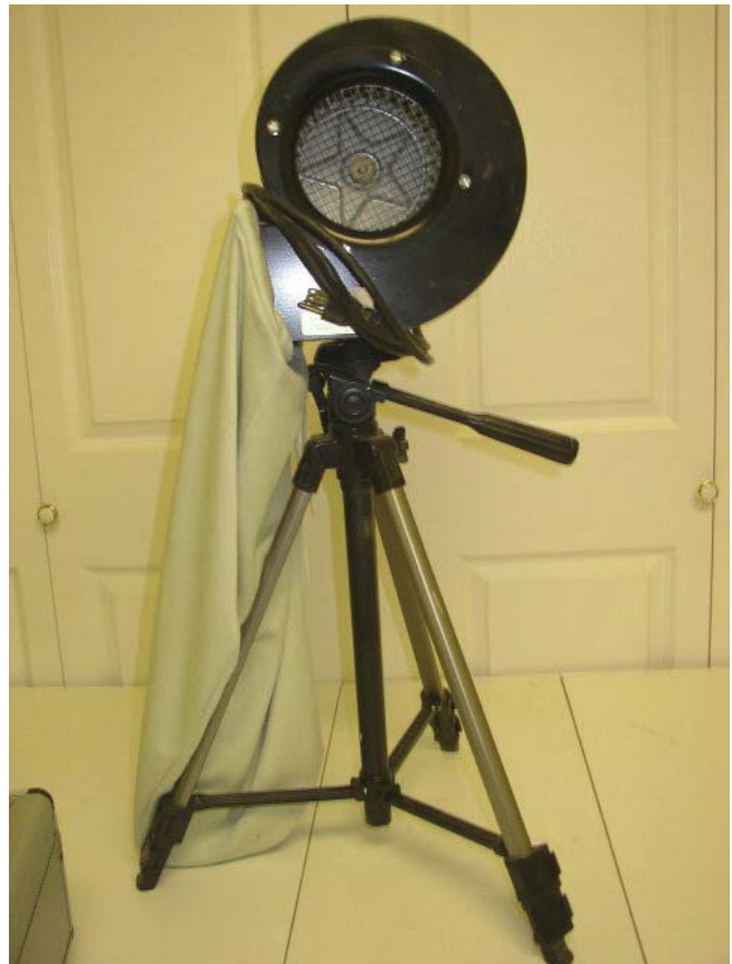
Shown above is a freestanding tripod mounted dust collector.
